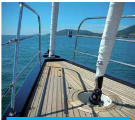
Flush-deck hydraulic furlers with spherical fulcrum - 125'
