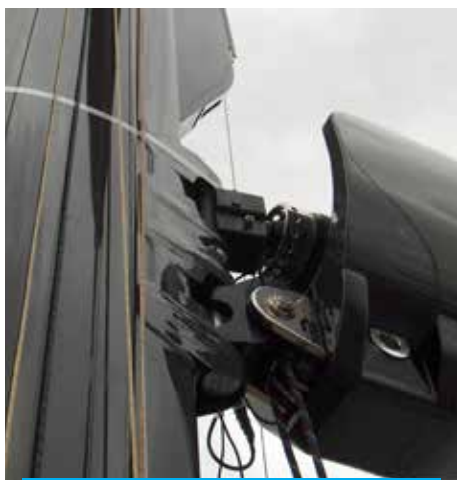
BFBMESS in-boom furling mechanism
